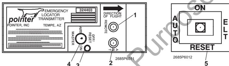
Figure 1. Pointer Model 3000-11 Emergency Locator Transmitter
