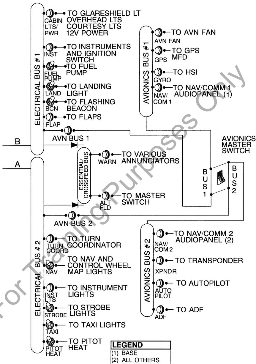
Figure 7-7A. Electrical Schematic (Serials 17280984 and On)
