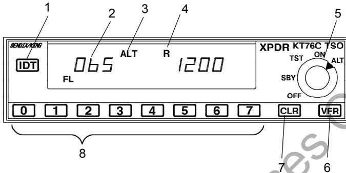
1. IDENT BUTTON (IDT) - When depressed, selects special identifier pulse to be transmitted with transponder reply to effect immediate identification of the airplane on the ground controller's display. ("R" will illuminate steadily for approximately 18 seconds. Button illumination is controlled by the avionic light dimming rheostat.
