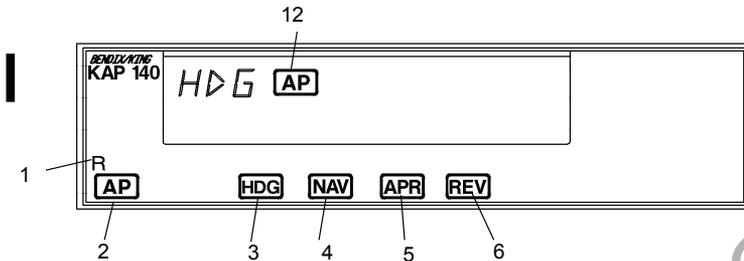
1. ROLL (R) AXIS ANNUNCIATOR -- When illuminated, indicates a failure in the roll axis and prevents engagement or disengages the autopilot.
